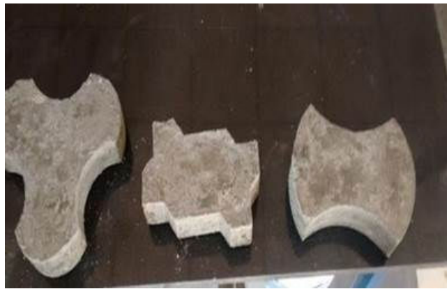
(c) Paver blocks after curing (MILANO, ZIGZAG, BASIL)
