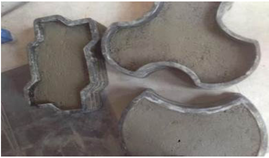
(a) Paver blocks after being molded
