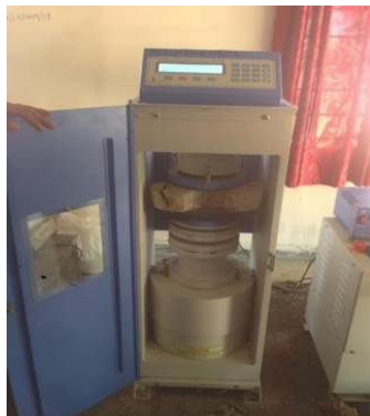
Compressive strength testing machine
